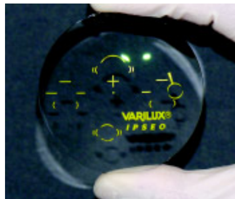
FIGURE 3 A finished Varilux® Ipseo™ progressive lens, complete with the markings necessary to block the lens for edging to the frame shape.
