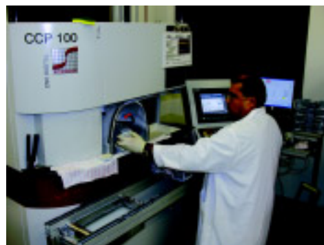
FIGURE 2 The complex surface of a freeform-generated lens requires special computer-controlled polishing to ensure the integrity of the surface is maintained.
