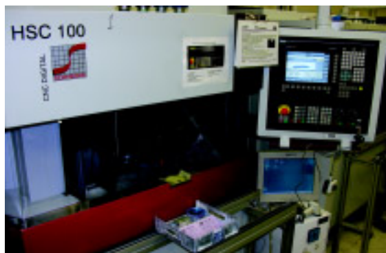
FIGURE 1 Freeform generators produce complex lens surfaces, such as those required for patient-customized progressive lenses.
